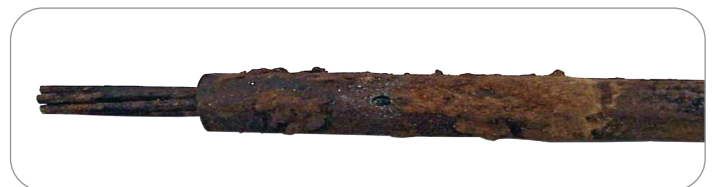
Figure 7 – Two-stage steel barrel, corroded due to insufficient compound
