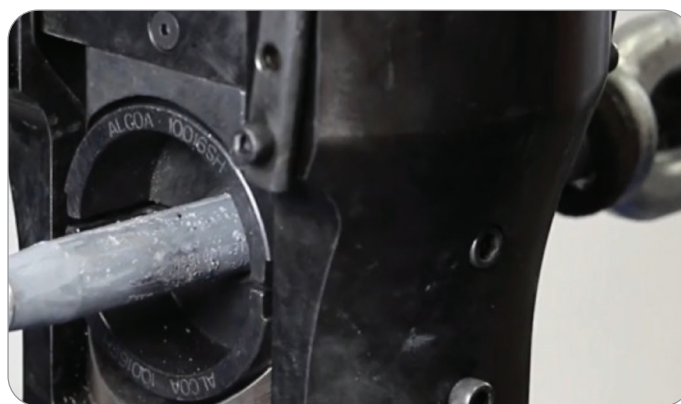
Figure 1 – Steel eye barrel compression for a two-stage fitting
