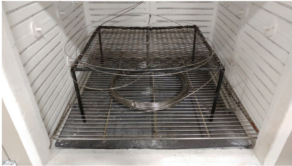
Figure 7: Cable configuration inside oven
