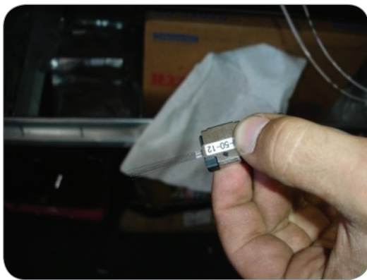
Photograph 13—SWR Ribbon Aligned into Splicing Fixture
