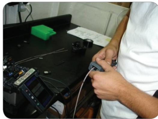
Photograph 14—Thermal Stripping of SWR
