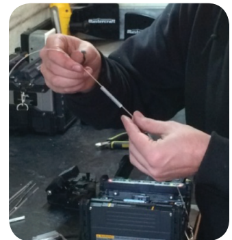
Photograph 16—Finished Mass Fusion Splice of SWR
