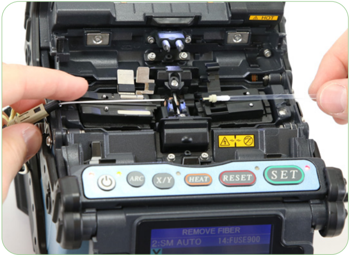
Splicing a FUSEConnect ST Connector
