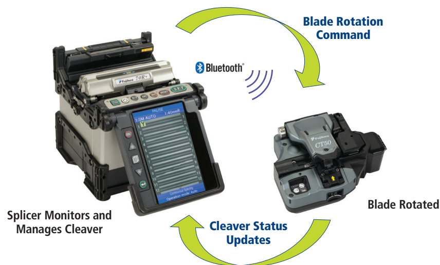
Figure 14—Cleaver Blade Rotation Management by 70R+ Splicer via Bluetooth
