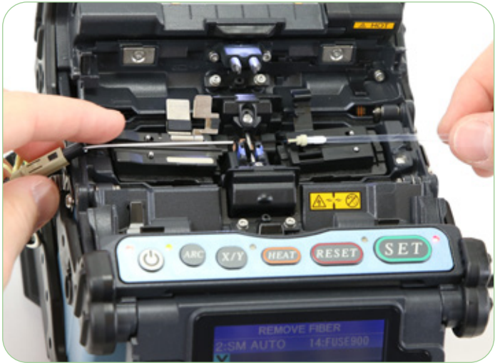
Splicing a FUSEConnect ST Connector
