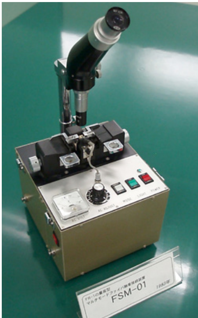
FIGURE 5: The 1st generation fusion splicer.
