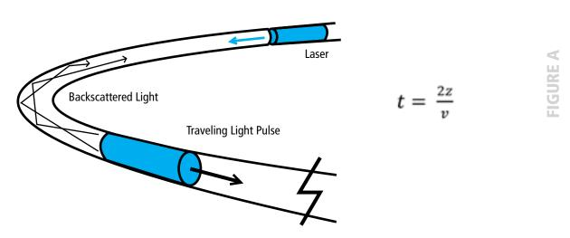
The time it takes for a pulse to travel down a length of the fiber and return to the sensor is referred to as the time of flight. The time of flight (t) of the pulse is proportional to the distance and speed it travels.
