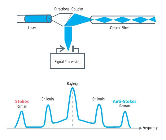
When DTS was first used, several limitations slowed enthusiasm for the technology. Many of these limitations have already been overcome. Fiber temperature ratings have drastically increased, up to 700°C. Optical fibers susceptibility to Hydrogen darkening has been delayed if not prevented through the use of hydrogen scavenging protective compounds, hermetic carbon coatings and improved glass chemistry. Fiber comes in much longer lengths and at much lower costs.
