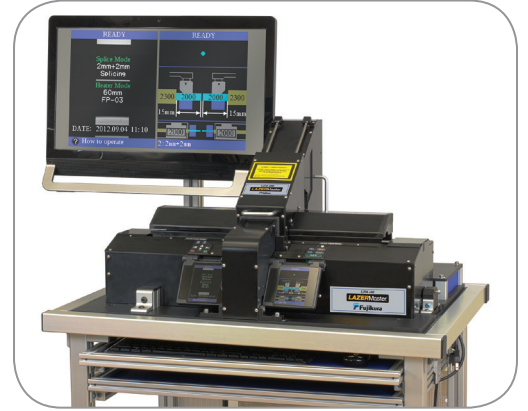
Fig. 10. Fujikura's LZM-100 glass processing station for fiber diameter ranged from 5 \mu m to 2.3 mm, tapering length up to 130 mm, and fiber melting temperature ranged from 100°C to more than 2,000°C.
