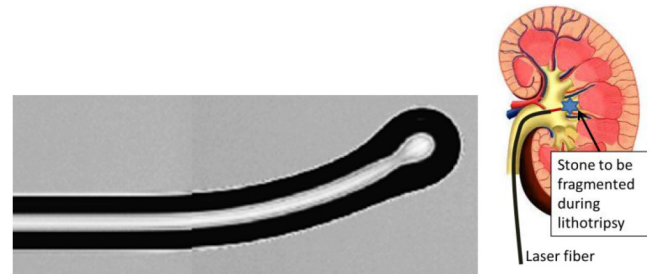
Fig. 9. 125 \mu\text{m} SMF28 with bent lens ( D = 150 \mu\text{m} , d_1 = d_2 = 125 \mu\text{m} , L = 400 \mu\text{m} , 2w_{02} = 20 \mu\text{m} , \phi = 30 \text{ deg} ). The ball lens picture was taken and stitched automatically by Fiber Processing Software for PC. The entire lens fabrication process is about 1 minute and fully automated.
