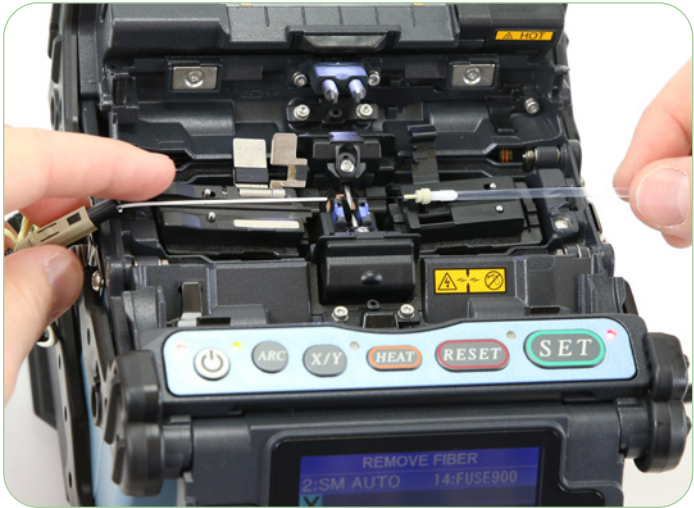
Splicing a FUSEConnect ST Connector
