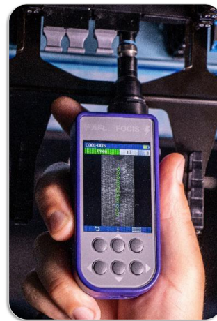
Figure 3: Multi-fiber inspection tools support MPO connectors
