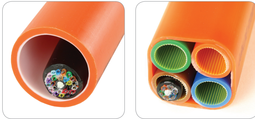
Figure 5 —The traditional 288-fiber loose tube, whether being air-jetted or pulled into the HDPE duct, requires a minimum duct size of 1" (left photo). In the photo on the right, the smaller LMHD 288-fiber cable can be installed via air-jetting into a 4-way micro-duct where each micro-duct has a 14 mm (0.55") ID. This 4-way micro-duct has the same overall size as the single HDPE duct. This means that total of four LMHD 288 fiber cables can be installed in the same pathway space that can support only one traditional loose tube cable.
