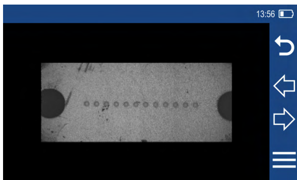
FIGURE 11: Image of MPO endface with dirt and debris.
