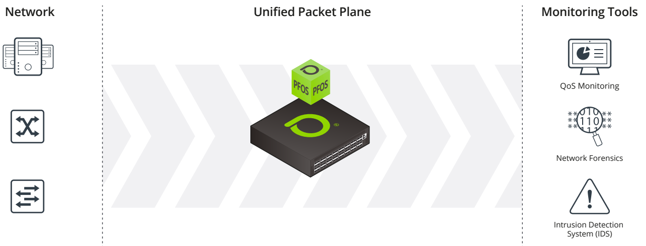
Figure 1: The NETSCOUT unified packet plane powered by PFOS (Packet Flow Operating System) logically separates the network from the monitoring systems.
