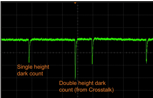
Figure 21. Oscilloscope Shot Showing Dark Counts
